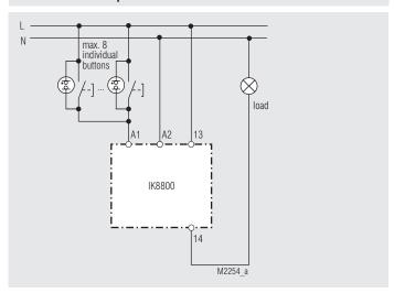
This circuit can be used with up to 8 illuminated pushbuttons.
