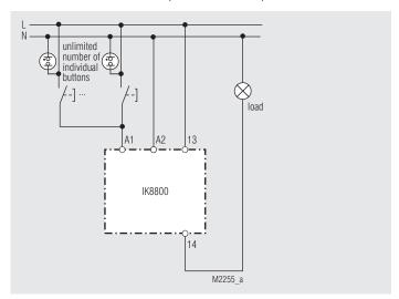
With this circuit it is possible to connect as many illuminated pushbuttons as required to a remote switch.
